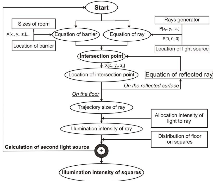
**Fig. 3:** Block diagram of the program
