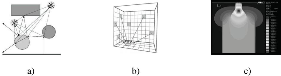
**Fig. 1:** a) Ray-tracing , [4], b) Radiosity, c) Illumination intensity distribution in the light conductor (obtained by means of applying the R-FEM method) [2].
