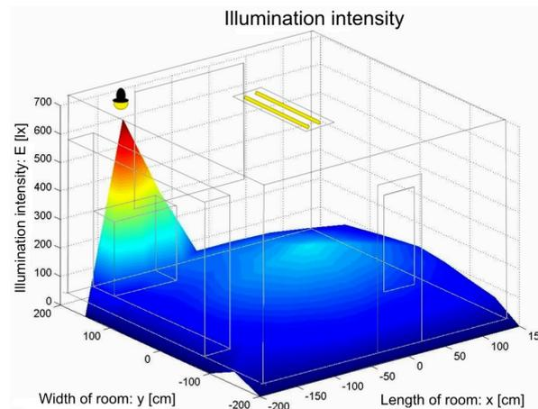
**Fig. 2:** Illumination intensity distribution in the room
